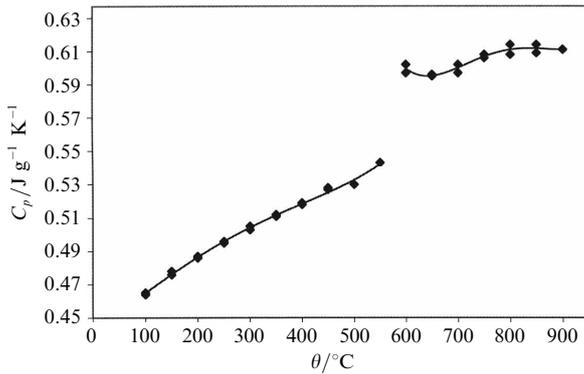
**Figure 6.** Specific heat capacity of Nimonic 75 cut from the 25 mm diameter stock.
