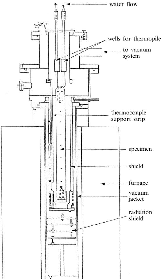
Figure 1. The NPL standard long-bar apparatus.
