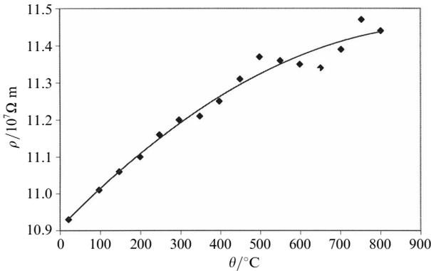
**Figure 4.** Electrical resistivity of Inconel 600 cut from the 25 mm diameter stock.
