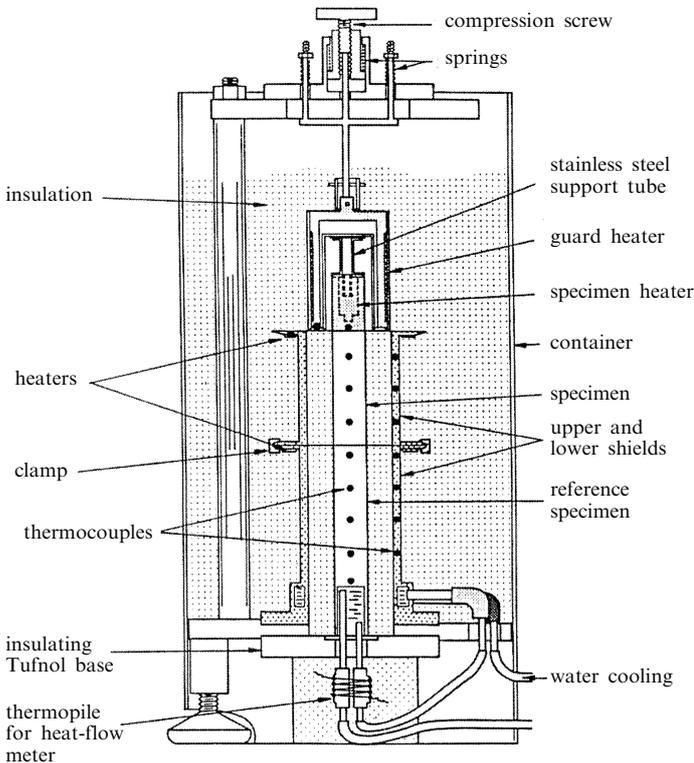
**Figure 2.** The NPL short-sample apparatus.
