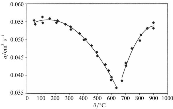
**Figure 5.** Thermal diffusivity of 430 stainless steel cut from the 25 mm diameter stock.
