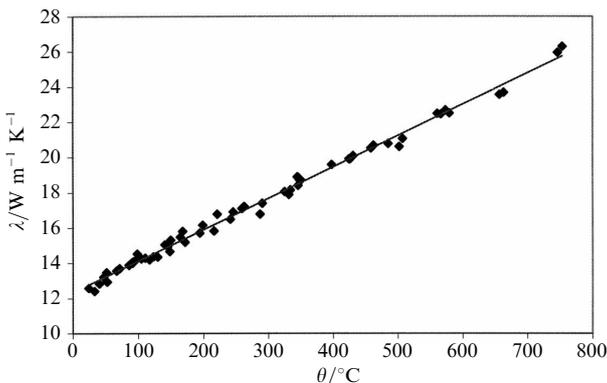
**Figure 3.** Thermal conductivity of 310 stainless steel specimens cut from the 25 mm diameter stock.
